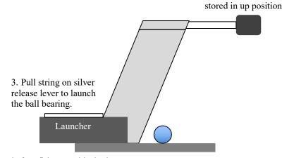
2. Just before firing, use black plunger to load the ball into the launcher and compress spring to firing position.
